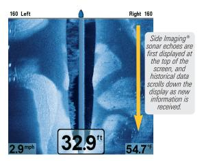
The main benefit of Side Imaging® sonar to anglers is that it provides an overall survey of a large area of water. This gives you a better understanding of the bottom topography and how structure is oriented for more efficient fishing.
