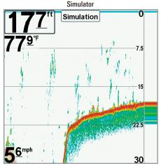
We recommend going through this manual while using the Simulator, since all of the menus function and affect the display in the same way as they would in Normal operation. Any menu changes you make will be saved for later use.
