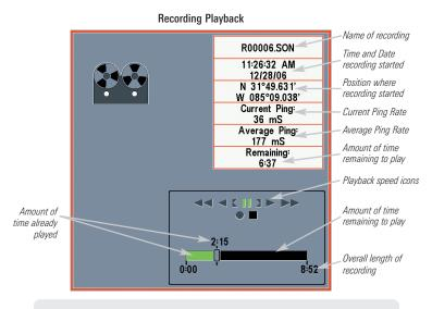
When you save screen snapshots and recordings to an SD card, a .DAT (or a .TXT) file is created for every .PNG screen snapshot, and a .TXT file is created for every recording folder. These data files are required for viewing the screen snapshots and recordings on your control head, so don't delete these files.
