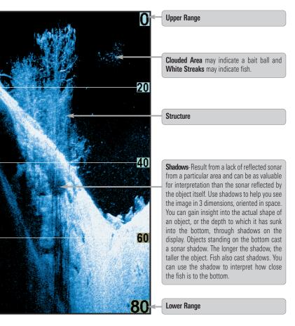
either device is connected to the 500 Series™ Fishfinder. If both devices are connected.
