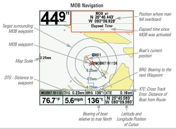
**Cancel MOB navigation:** From the Navigation X-Press<sup>™</sup> Menu, select Cancel MOB, and press the RIGHT Cursor key. Canceling MOB navigation removes the route and any waypoints created using the GOTO key but does not remove any saved routes from memory.
