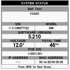
Self Test displays results from the internal diagnostic self test, including unit serial number, Printed Circuit Board (PCB) serial number. software revision. total hours of operation, and the input voltage.
