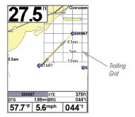
Add a Waypoint Target: Open the Waypoint Management dialog box and select a Waypoint. Press the RIGHT Cursor key, and select Target. Press the RIGHT Cursor key.
