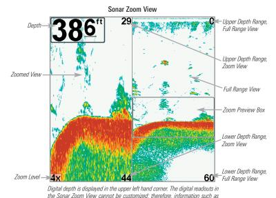
water temperature and voltage are unavailable in the Sonar Zoom View.
