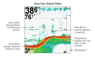
Use **Bottom View** to select the method used to represent bottom and structure on the display. See *Sonar Menu Tab* to set the Bottom View.
