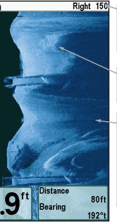
Side Imaging® Range - Images shown on the right side of the screen are located on the right side of your boat, and images shown on the left side of the screen are located on the left side of your boat. In this illustration, the sonar is pinging 150 feet on each side.
