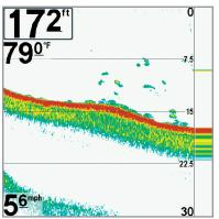
Structure ID® represents weak returns in blue and strong returns in red when Sonar Colors is set to Original. If the Sonar Colors palette is changed, the Structure ID® will display the strongest return as specified by the palette. See Sonar Menu Tab: Sonar Colors for more information.
