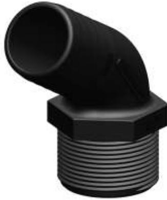
TruDesign Tails are moulded from a glass reinforced nylon composite. High strength, high-modulus glass fibres impregnated into the nylon provides dramatic strength, stiffness, toughness, and dimensional stability. TruDesign Tails eliminate the corrosion and electrical bonding problems associated with metallic fittings. The Tails are designed for twin hose clamps, and to not crush under high load conditions.
