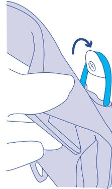
5 The back of each product has loops in each corner. Hang the top two cord loops over the hooks and stretch the two bottom elastic loops over the lower hooks.
