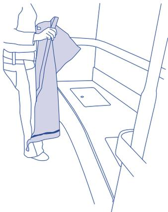
2 Place the bunknet with silver side up. Check if final height of the bunknet is ok.
