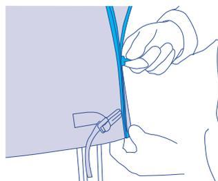
3 Fix the cover around the mast with the Velcro straps. Fasten with the buckle.
