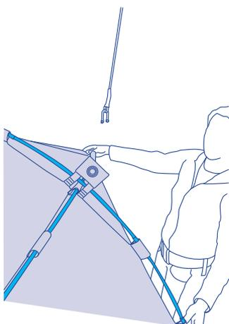
6 Fix its position using the corner cords attached to the railing.
