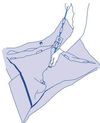
4 Tension the batten and force the tip in the corner pocket.
