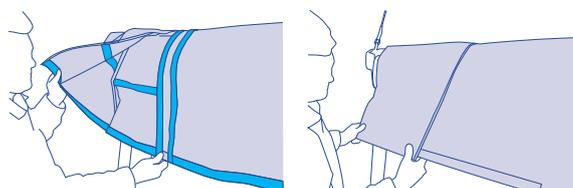
5 Attach the rear end of the cover with cord to the end of the boom.
