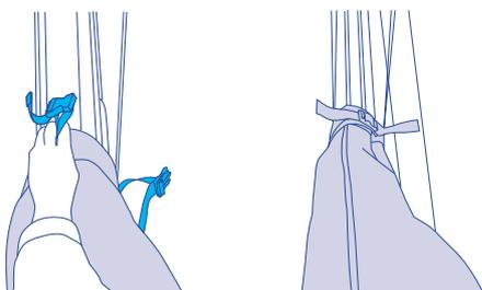
4 Define cover length to fit your boom with the separate flap at the rear. Adjust double layer of the flap and fix it with Velcro.
