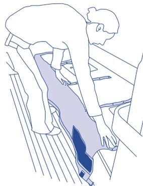
3 Choose a hole in the webbing closest to the front edge of the seat. Fix 5 x screw through the webbing.
